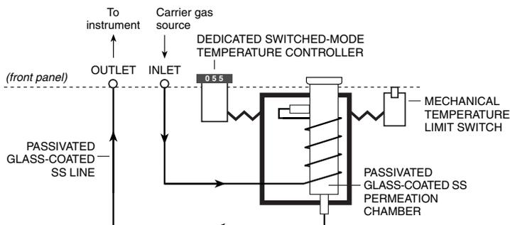
**Figure 1:** Dynacalibrator Model 150 schematic
