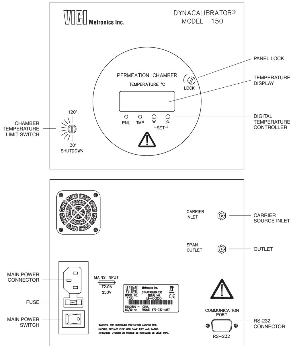
Figure 2: Dynacalibrator Model 150 front and rear panels
