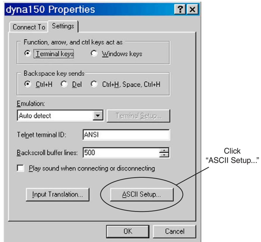
10. Click “ASCII Setup” and set the parameters as indicated below.
