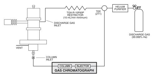
Figure 3: Gas connections for a PD-D2-IM system
