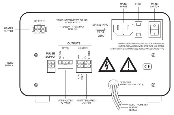
**Figure 2:** Controls and connections on front (top) and back panels of the control module
