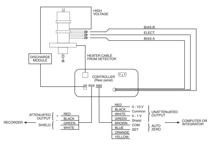
Figure 4: Electrical connections
