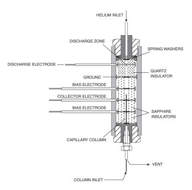
Figure 1: Schematic of the D-2-IM detector
